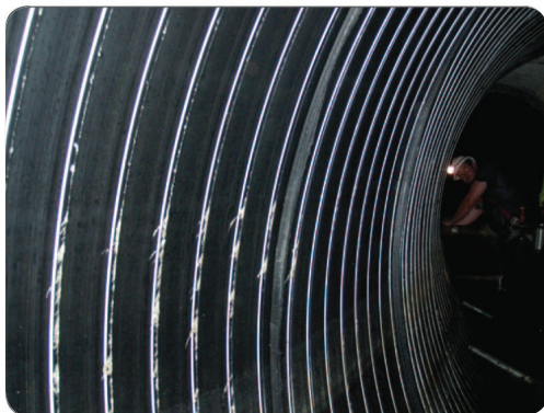
New configuration of profile strip now allows Ribline to be wound and slipped around.
