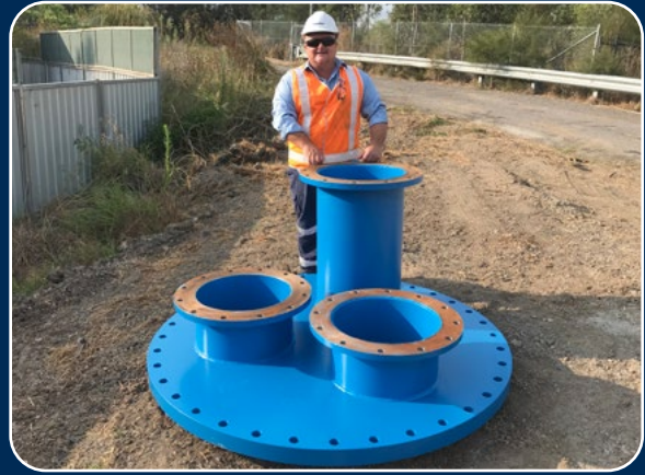
A custom-built manifold to allow three liners to be installed at once.
