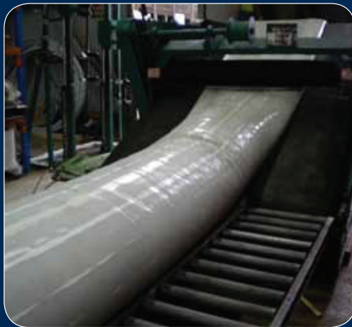
The Interline CIPP resin impregnation process is performed inside controlled conditions
