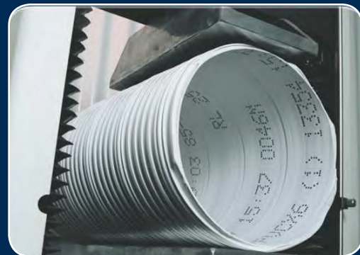
Strength testing of the Expanda liner.
