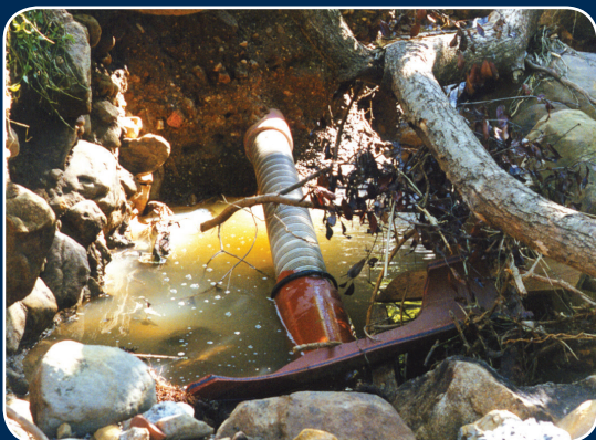
Proven strength: Floods smash the clay pipe but the Expanda liner remains intact.
