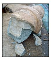
Picture 11: Pipe filled with concrete
