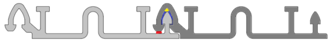
Figure 6: Rotaloc bend profile strip cross section with the "loop" that allows continuous lining around a bend
