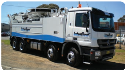
The Super 2000 is capable of cleaning pipes from DN150 to DN1500.
