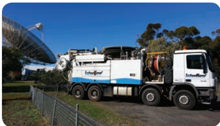
The Super 1000 is capable of cleaning pipes from DN150 to DN750.
