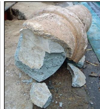
Picture 11: Pipe filled with concrete
