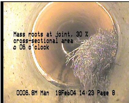
Picture 4: Roots growing through a crack or joint in the pipe
