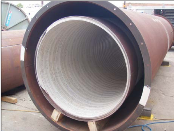
Picture 1: Assembly for the unsupported liner test, prior to placing the end sealing bungs. The Rotaloc liner is located centrally in the cylindrical pressure vessel
