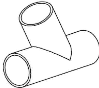
Figure 1: 3D view of the CIPP lateral junction sealing fitting
