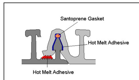
Figure 2: Rotaloc lock configuration
