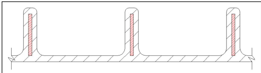
Figure 3: General arrangement of Ribline cross section showing steel encased in the polyethylene
