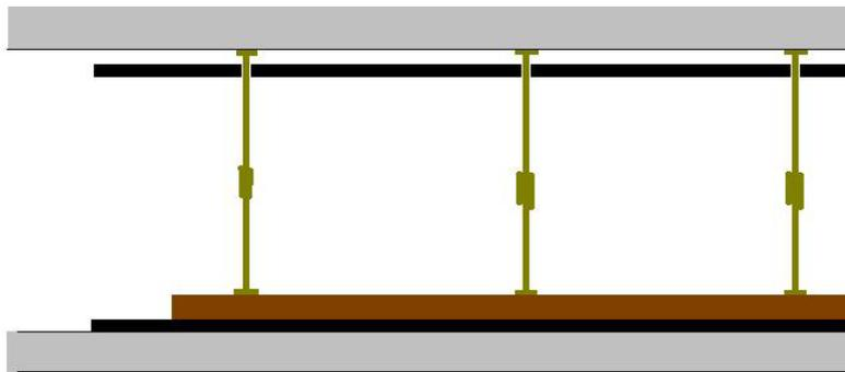
*Figure 6: Temporary scaffold access to lining chamber in gully*
