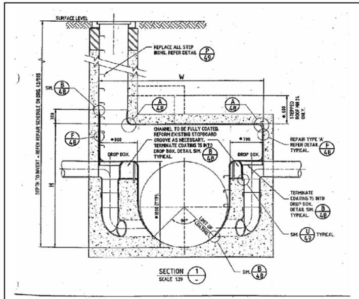
Figure 5: Access chamber detail at Coogee
