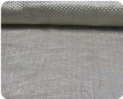
Fibreglass matting gives Interpatch high strength
