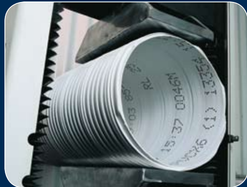
Strength testing of the Expanda liner.
