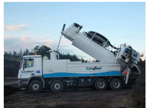
The silt and debris that is collected from the pipe is disposed of at a suitable waste facility.
