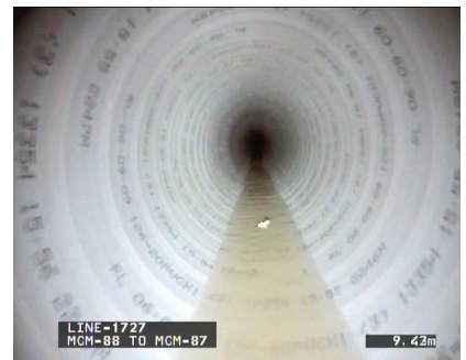
Post lining CCTV shot. Expanda can be installed in pipes with missing wall sections and the new pipe is circular in cross-section.
